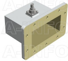
430WCASM Right Angle Rectangular Waveguide to Coaxial Adapter 1.7-2.6GHz WR430 to SMA Male
